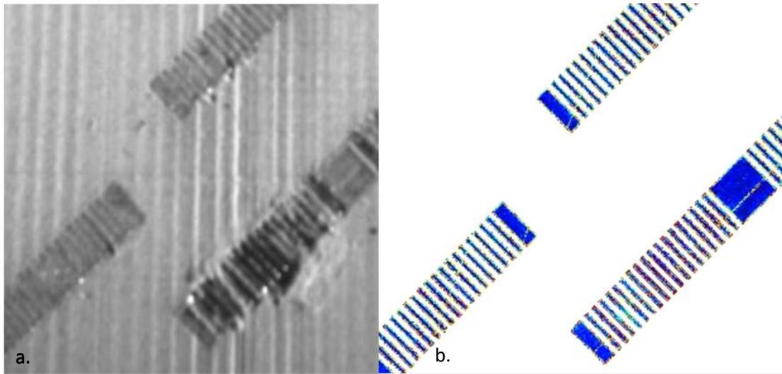
Figure 5: EOS powder bed image layer 314. b, TEP™ Sigma Scan Viewer layer 314
