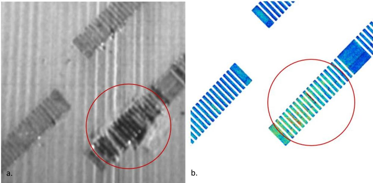
Figure 4: EOS powder bed image layer 314. b, TEP™ Scan Viewer layer 314
