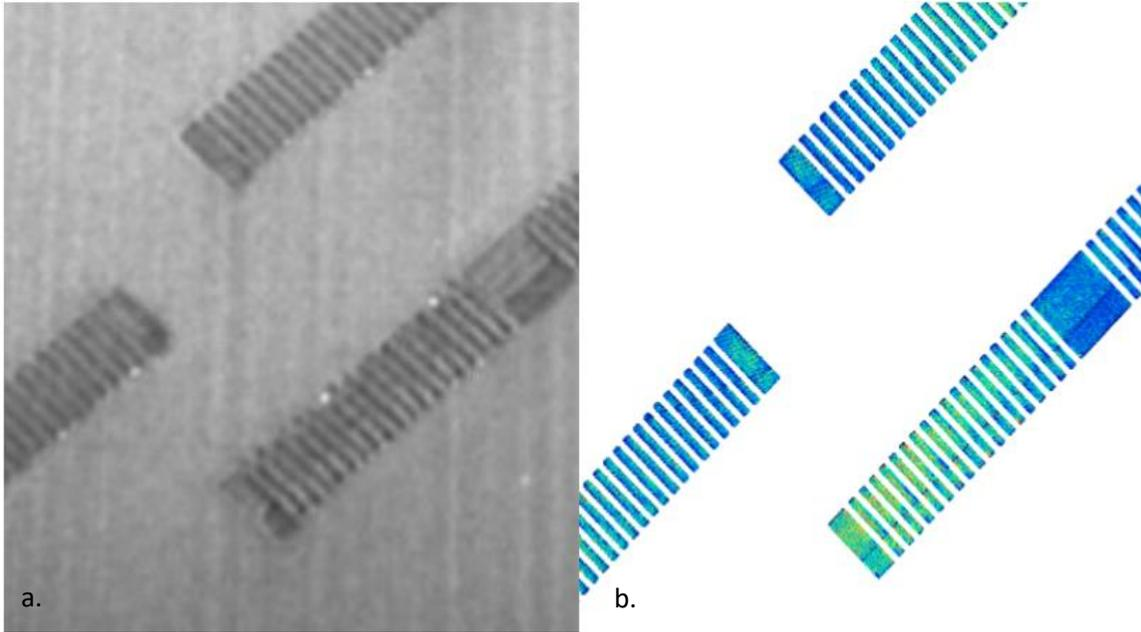
Figure 3: a. EOS powder bed image layer 50. b, TEP™ Scan Viewer layer 50
